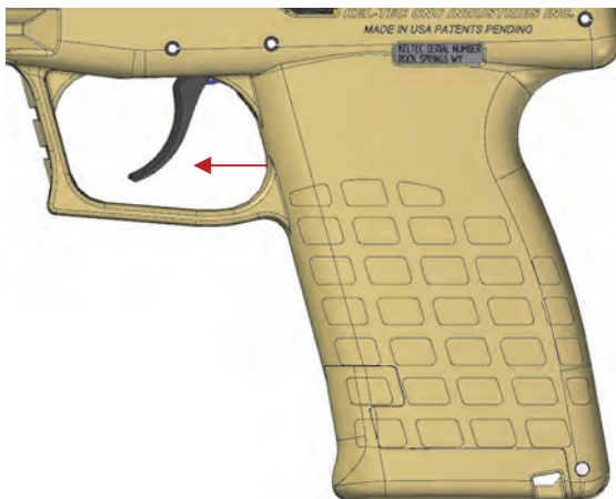
Figure 11. Push Trigger Forward to Disassemble
